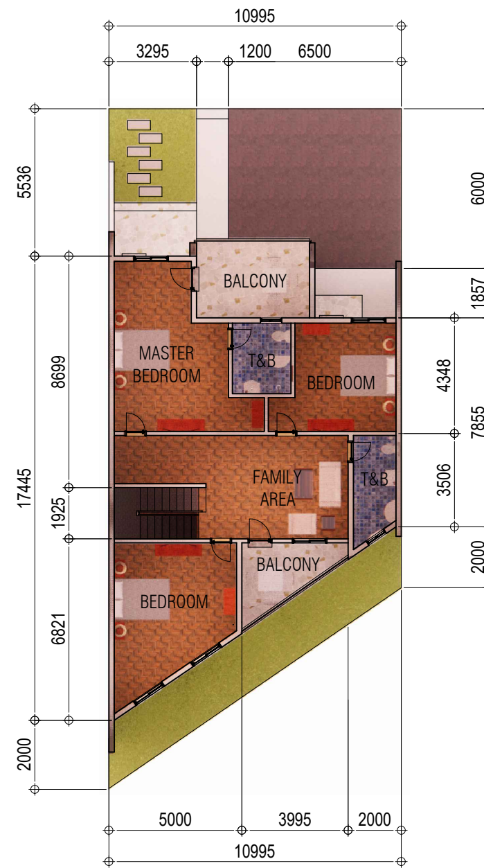
CORNER LAYOUT OF TOWNHOUSE SECOND FLOOR PLAN SCALE 1:50
